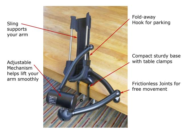
The NAS-Zero supports the weight of the user's arm in a sling, enabling them to move their arm back and forth freely using their own muscle power. It is usually supplied with a fixed bracket system for clamping to a sturdy table. It can also be attached to the back of a wheelchair or to a separate floor stand.
