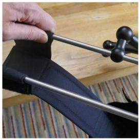
Slide off the front. Rubber ends inside should remain inside the sling
