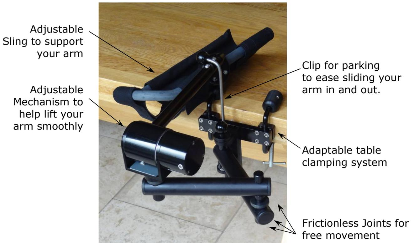
The NAS-Zero supports the weight of the user's arm in a sling, enabling them to move their arm back and forth freely using their own muscle power. It is usually supplied with a fixed bracket system for clamping to a sturdy table. It can also be attached to the back of a wheelchair or to a separate floor stand.
