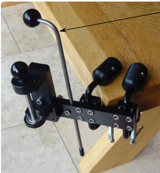
Clip for holding down the sling frame to enable sliding arm in and out.
