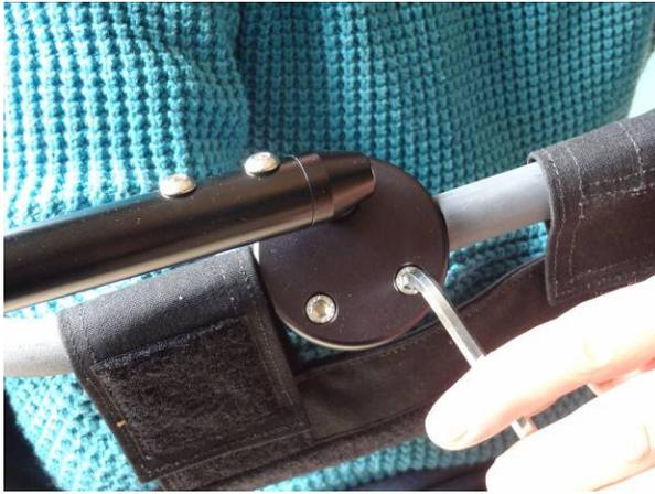
Loosen two screws in the Angled Joint and slide the frame to change the pivot position before retightening the screws. (The flexible tubing around the frame may need carefully cut).
