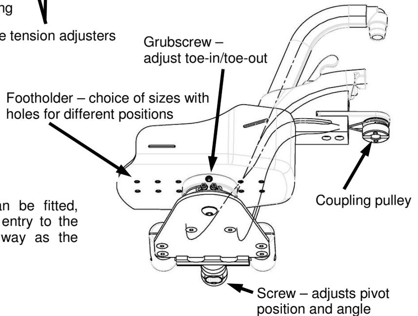
The steering footrest assembly can be fitted, swung out of the way for ease of entry to the chair and detached in the same way as the conventional footrest.
